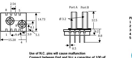
Connect between Gnd and Vcc a capacitor of 100 nF
