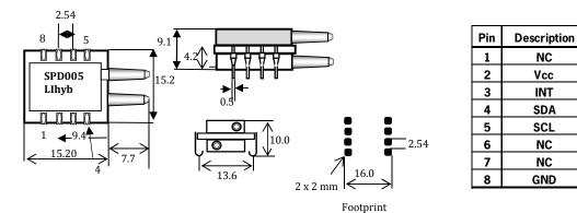
Use of NC pins will cause malfunction Connect between Vcc and Gnd a capacitor of 100 nF.
